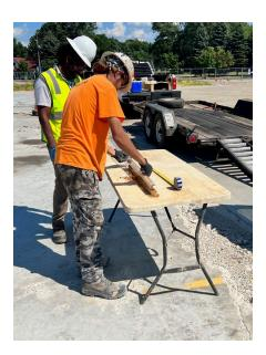
Tetra-Tech employees are evaluating a four-foot-deep sample of soil. Samples are collected from each one-foot increment of the section, placed into specimen jars, labeled, and sent to the lab to determine if volatile organic compounds and/or PCB containing material are present below the concrete floor.
