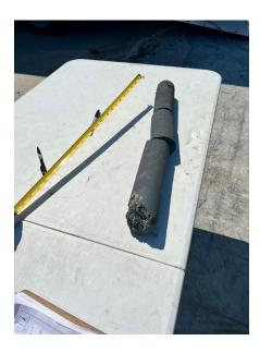
The core sample in this photo is visually inspected, measured, the sample location documented, and will be sent to a lab to determine the concentration of what is presumed to be PCB containing material. Samples are being taken at predetermined intervals and as deep as four feet. GPS equipment will be used to collect location data on each of the samples for future mapping of the location, depth, and concentration of the contaminants.
